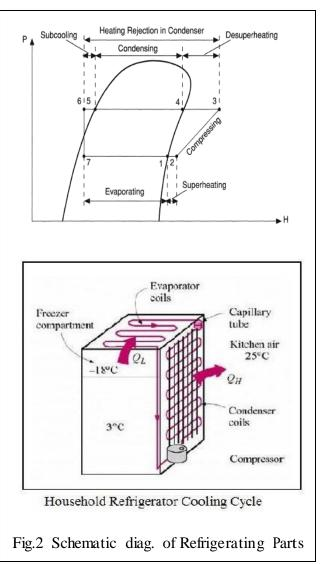
thin copper tubing made up of number of turns of the copper coil. When the refrigerant is passed through the capillary its pressure and temperature drops down suddenly.
